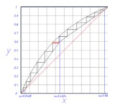
Figure 1: Graphical method - theoretical plate layers.
