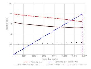
Figure 2: Load performance diagram for the rectifying section.
